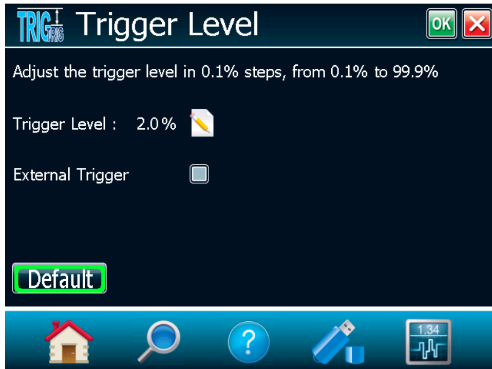
Fig. 2-17 Trigger Level window
