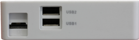
Fig. 7.3: View from the right. Left to right: micro-SD card connector, two USB type A female connectors
